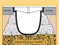
Always backfill with concrete with the grating fitted
