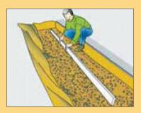
Dig Trench - compact GAP7, backfill and level
